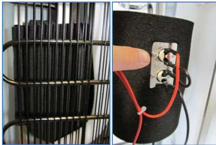
4. *Using a chopstick or screwdriver, depress the hot tank reset button (water should be hot in 30 minutes time, see figure below which pictures hole used to access hot tank reset button)*
